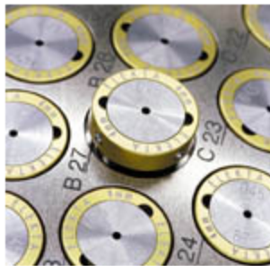
Collimators 4mm, 8mm, 14mm, 18mm depending on size needed to accurately target lesion
